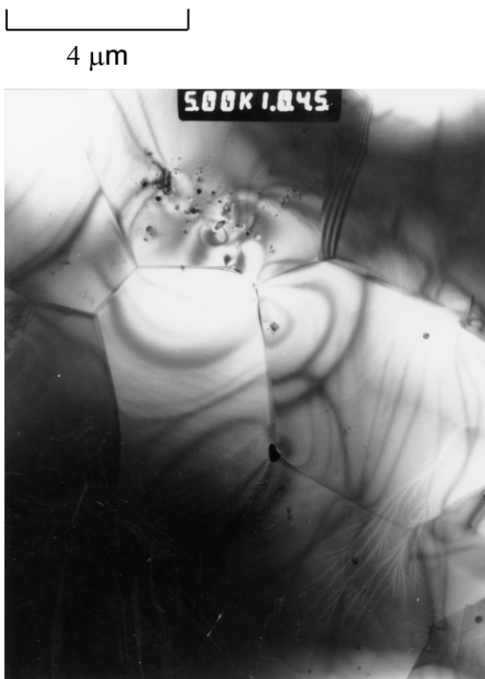
Fig. 9. TEM micrograph showing the typical microstructure of the RA207LS/ENEANanocomposite processed at high pH.
