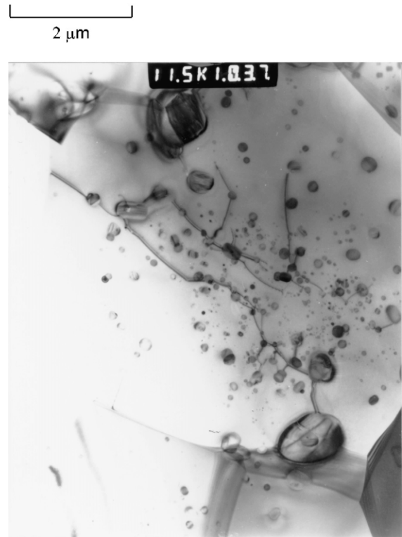
Fig. 19. TEM micrograph showing extensive sub-grain boundary formation in an RA207LS/ENEAnanocomposite processed at low pH.
