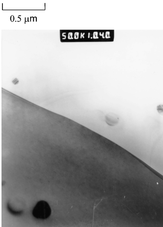
Fig. 14. High magnification TEM micrograph of an \text{Al}_2\text{O}_3/\text{Al}_2\text{O}_3 grain boundary in the RA207LS/ENE system processed at low pH.
