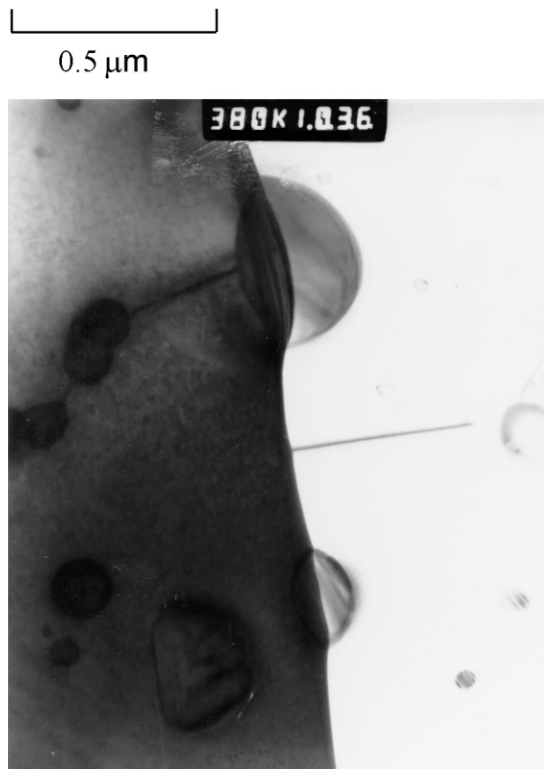
Fig. 8. TEM micrograph showing the effect of grain boundary silicon carbide on the morphology of the interface in an RA207LS/ENEANanocomposite processed at low pH. The presence of a sub-grain boundary is also evident.
