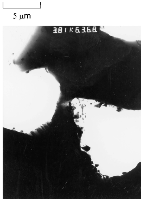
Fig. 11. TEM micrograph showing the typical microstructure of the CR15/UF15nanocomposite.
