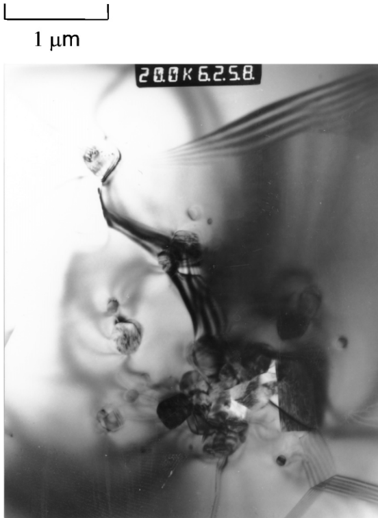
Fig. 13. TEM micrograph showing a small SiC cluster in an RA207LS/UF32 nanocomposite, showing absence of amorphous grain boundary phase(s).
