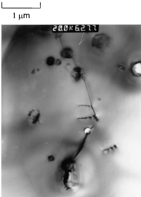
Fig. 18. TEM micrograph showing sub-grain boundary and associated dislocations in an RA207LS/UF45 nanocomposite.
