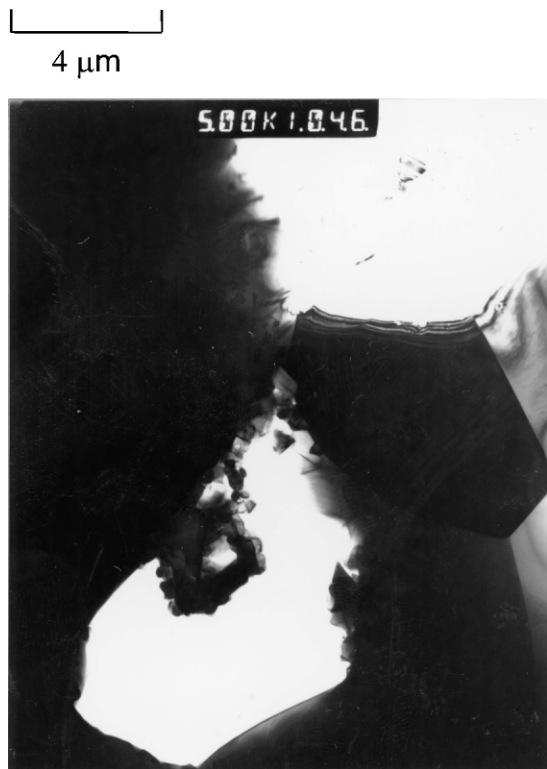
Fig. 10. TEM micrograph showing pore stabilisation by silicon carbide agglomerates in the RA207LS/ENEANanocomposite system processed at high pH. The remains of a silicon carbide agglomerate can be clearly seen in the pore in the top-left part of the micrograph.
