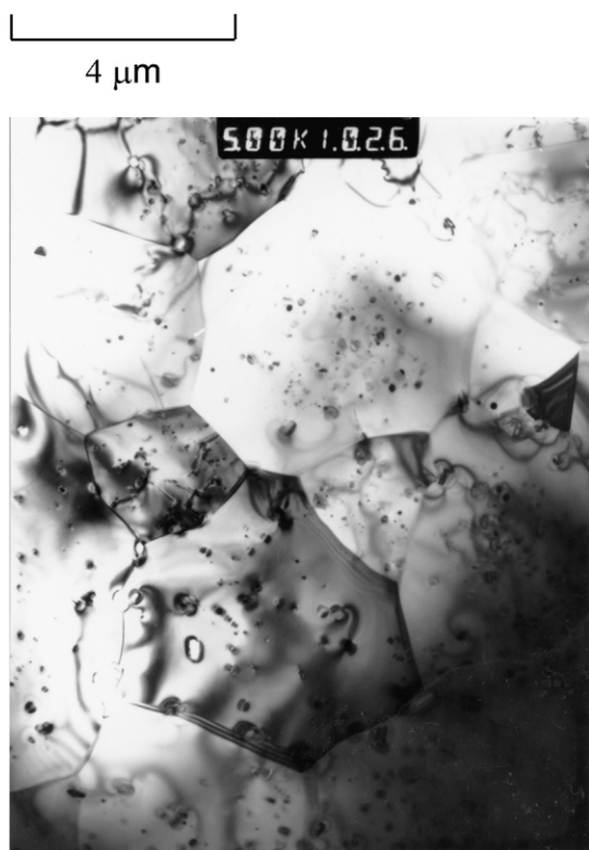
Fig. 7. TEM micrograph showing the typical microstructure of the RA207LS/ENEANanocomposite processed at low pH.
